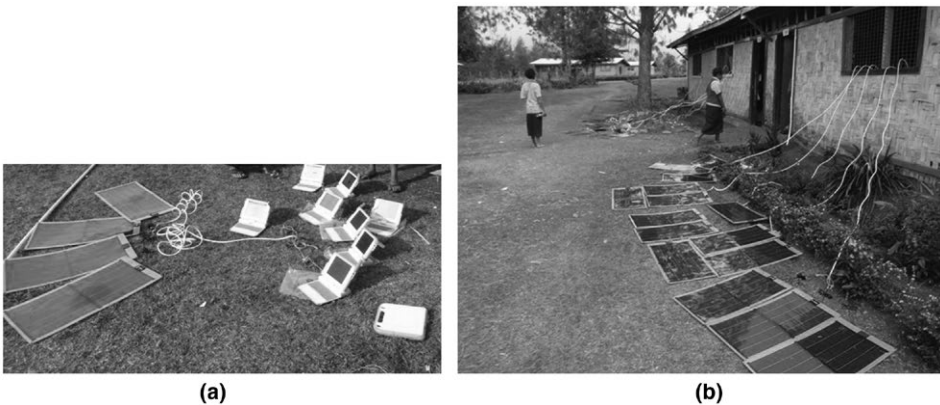
FIGURE 1. Examples of (a) thin-film solar panels and XOs, and (b) thin film solar panels used to power XOs inside a classroom (Source: https://wikieducator.org/OLPC_PNGSDP/Kisap ).
